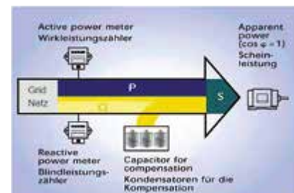
Fig.: Principle of power factor correction
