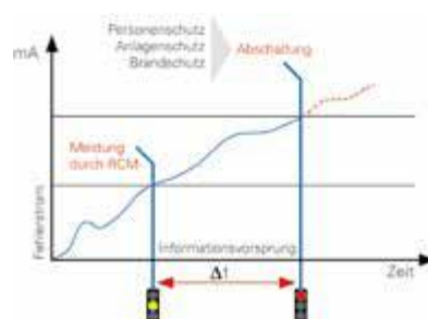
Fig. 1: Alert before switching off – An objective of residual current monitoring
