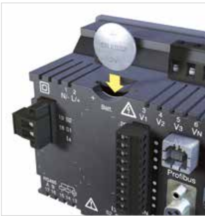
Fig.: Battery slot on the rear (UMG 96RM-CBM and UMG 96RM-P)
