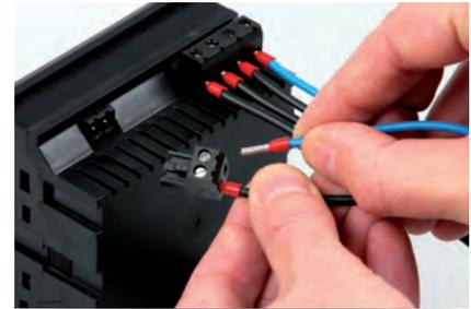
Fig.: Pluggable screw terminals for easy connection
