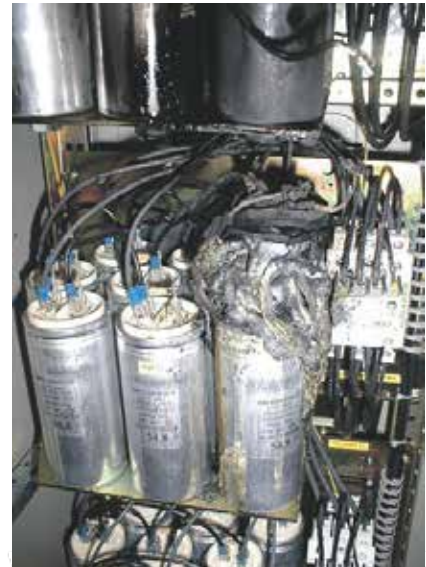
Fig.: Capacitors destroyed due to harmonics
